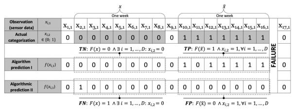
Figure 2. Four PdM model states in an example of 17 observations
